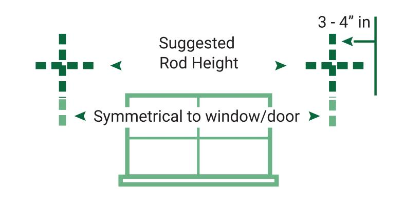
Place the center bracket mark at the exact center between the two end marks.
