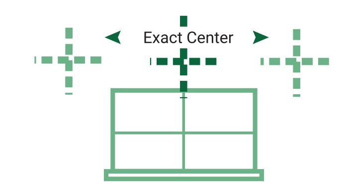
Make sure that all marks are level to the floor and placed in a straight line.
